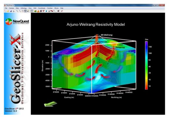
Figure 6: 3-D Resistivity Model Using GeoSlicer-X Software of the Arjuno-Welirang Geothermal Area
