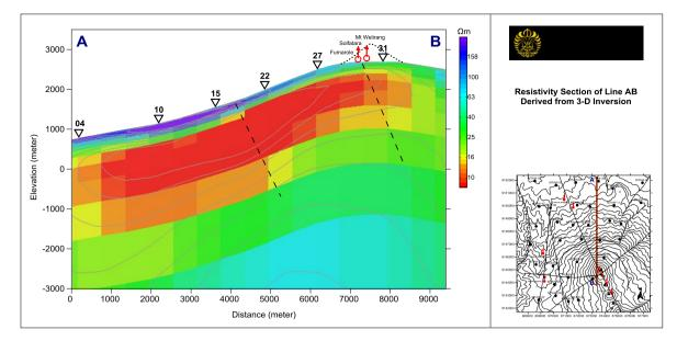
Figure 4: Resistivity Structure Derived from 3-D Inversion along Line AB of the Arjuno-Welirang Geothermal Area
