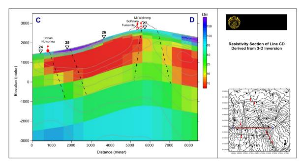
Figure 5: Resistivity Structure Derived from 3-D Inversion along Line CD of the Arjuno-Welirang Geothermal Area
