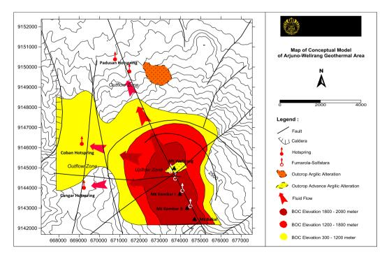
Figure 7: Conceptual Model Represented by BOC Elevation Contour and Hydrogeology Map of the Arjuno-Welirang Geothermal Area
