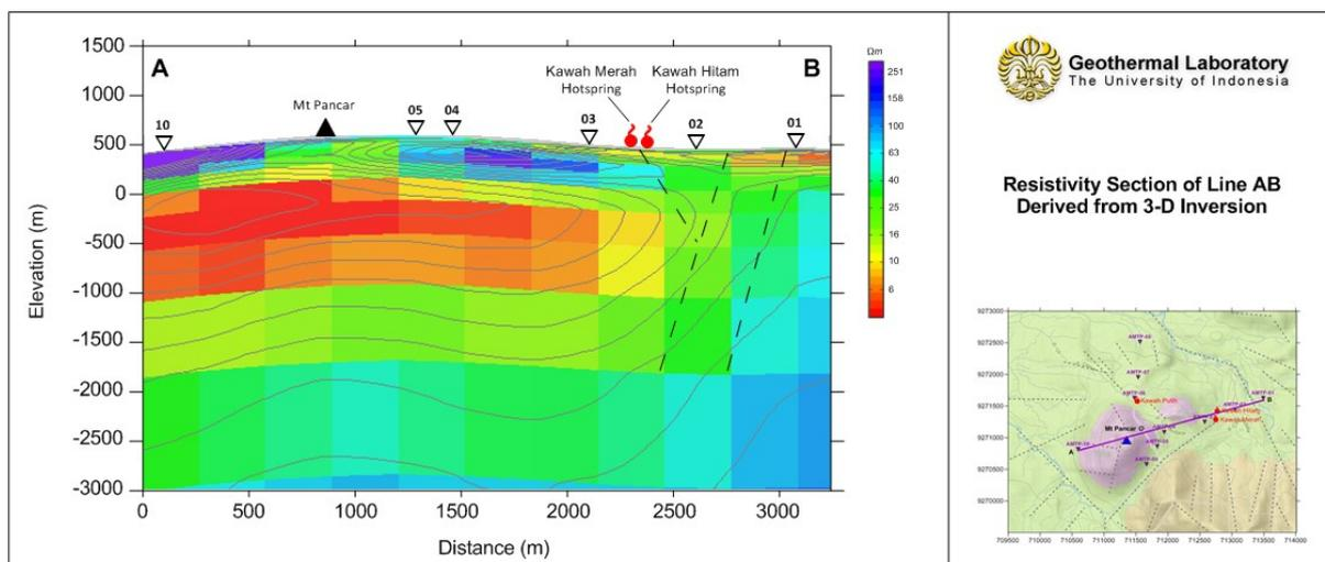
Figure 8: Resistivity Section Derived from 3-D Inversion of AMT Data (Line AB).
