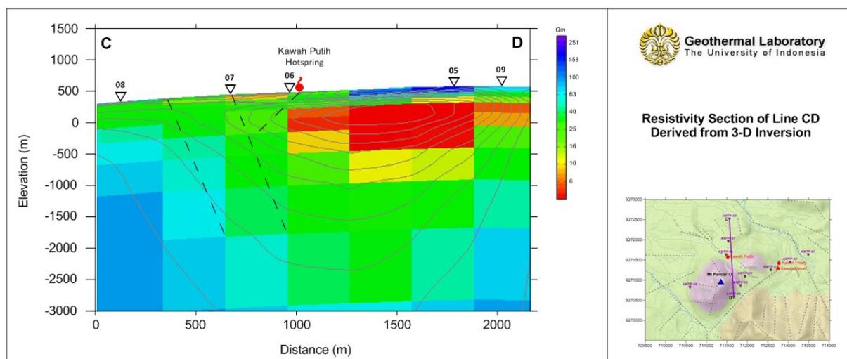
Figure 9: Resistivity Section Derived from 3-D Inversion of AMT Data (Line CD).
