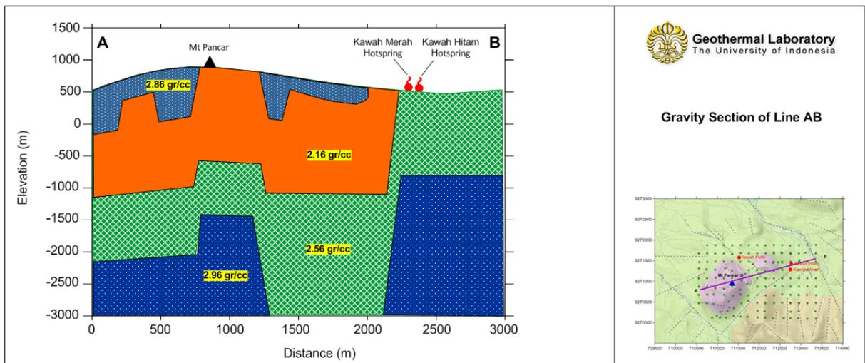
Figure 6: 2-D Gravity Modeling Along Line AB.
