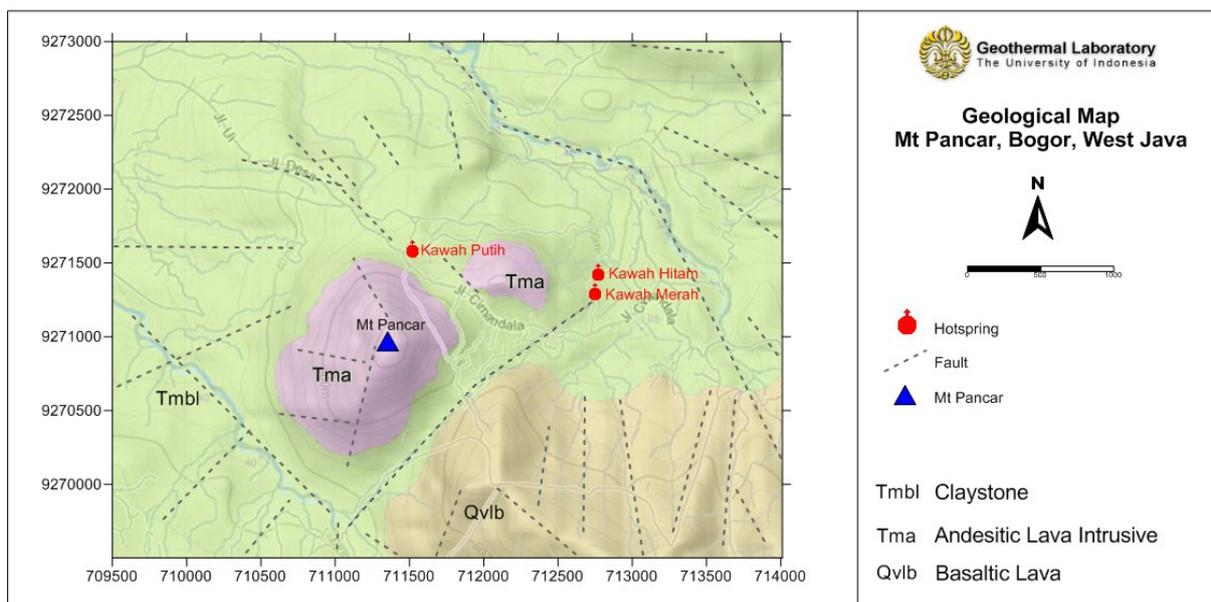
Figure 2: Geological Map of Mt Pancar Geothermal Prospect Area.
