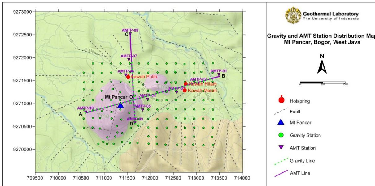
**Figure 3: Distribution of Gravity and AMT Measurement Stations in Mt Pancar Geothermal Prospect Area.**
