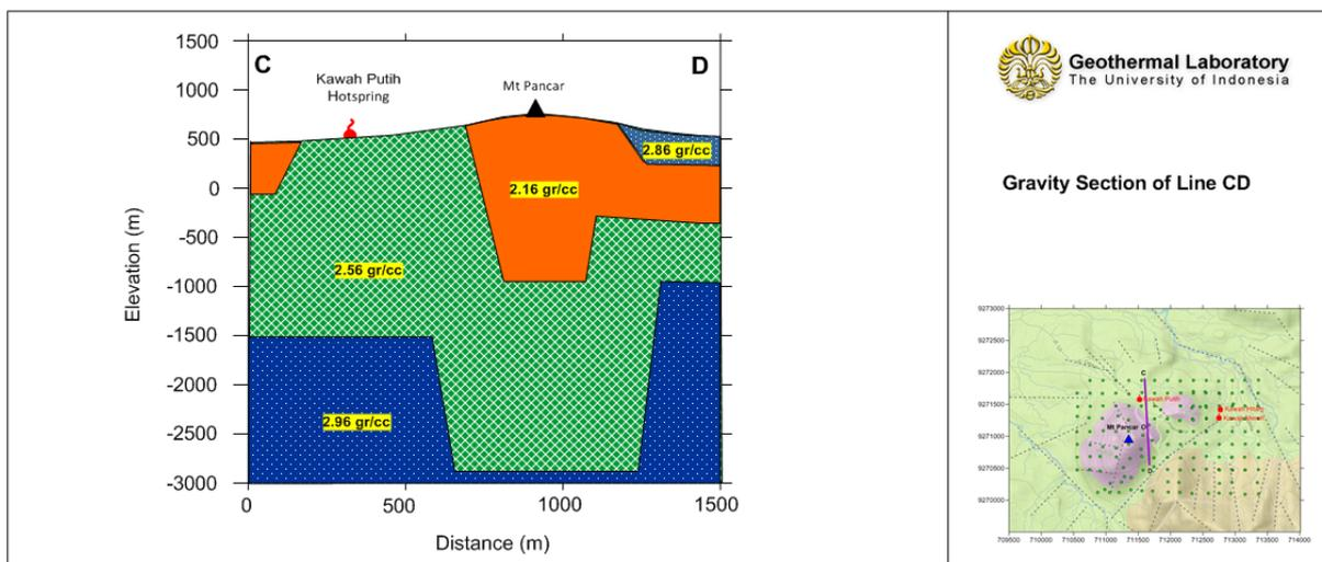
Figure 7: 2-D Gravity Modeling Along Line CD.
