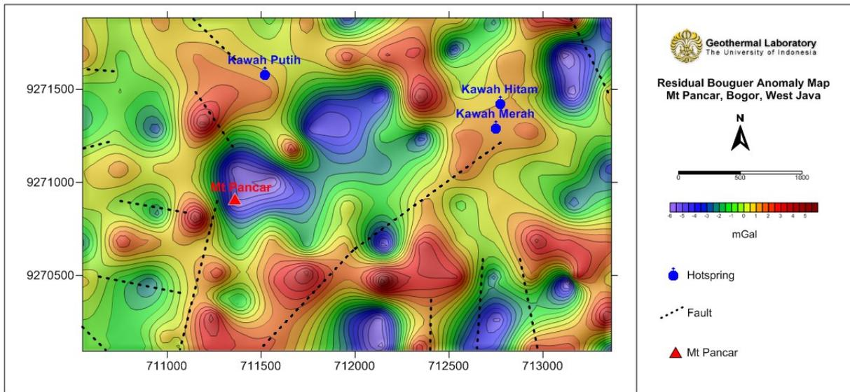
Figure 5: Residual Bouguer Anomaly (RBA) in Mt Pancar Geothermal Prospect Area.
