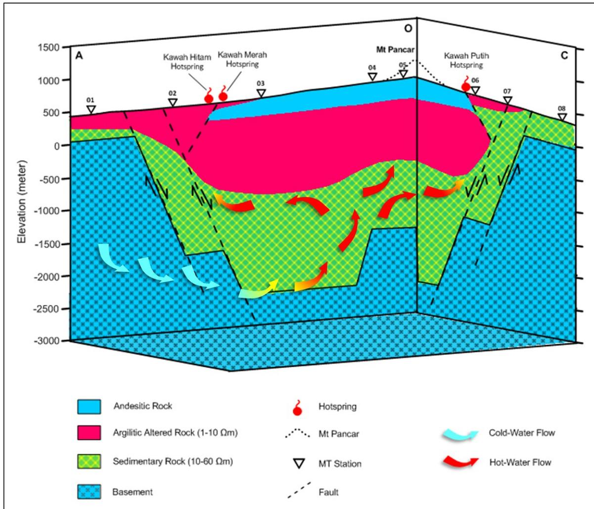
Figure 10: Conceptual Model of Mt Pancar Geothermal Prospect Area.
